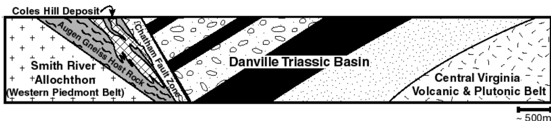
Figure 5-6. Vertical Cross-Section Showing Surrounding Geology and Approximate Ore Body Configuration
